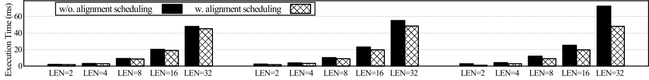
Fig. 10. Performance of GPU kernels evaluating various expressions. From left to right, the expressions are a+b+a , a+b+a+a+a , and a+b+a+a+a+a .
